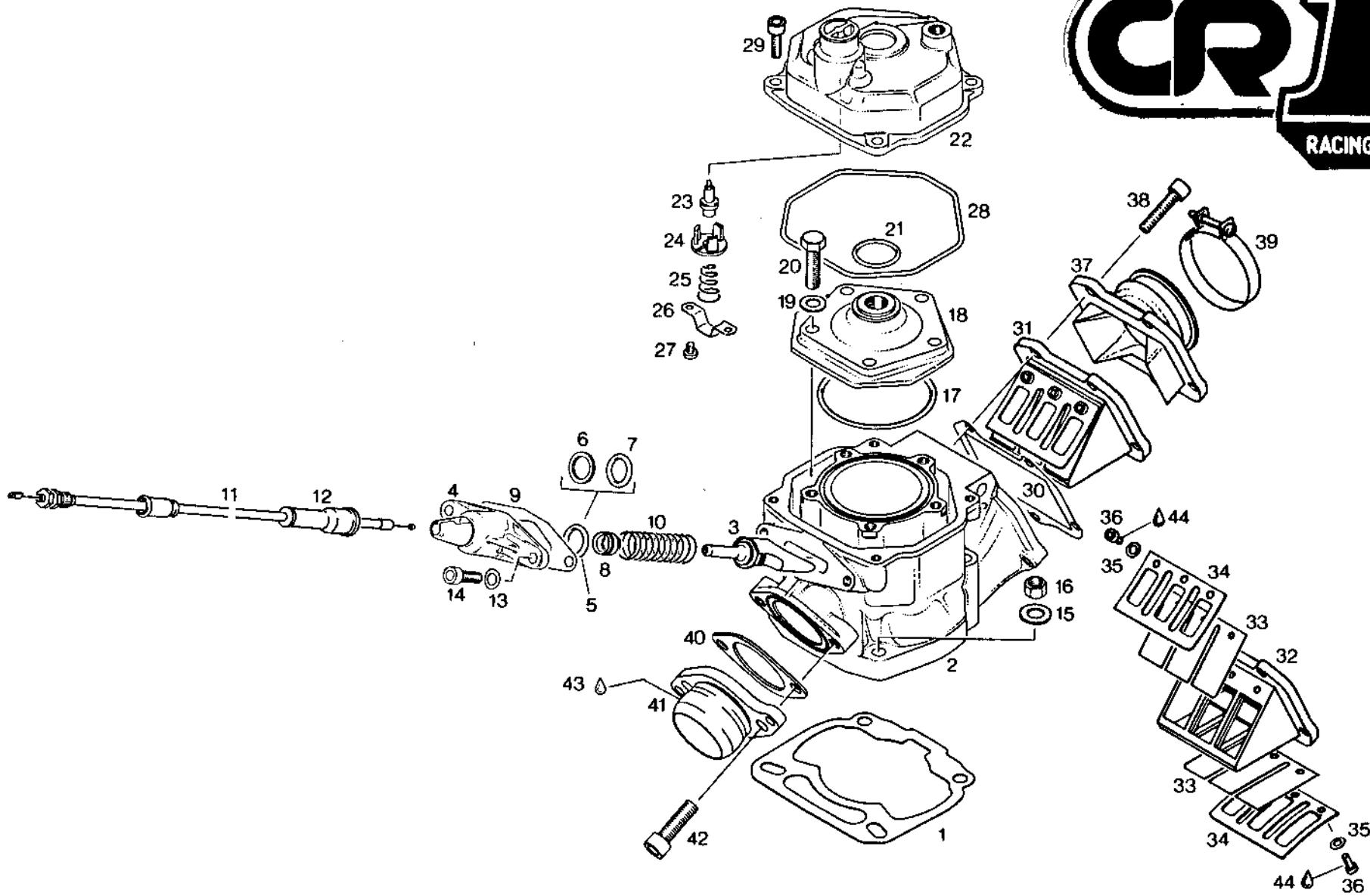
ZYLINDER, AUSPUFFSCHIEBER, ZYLINDERKOPFDECKEL
